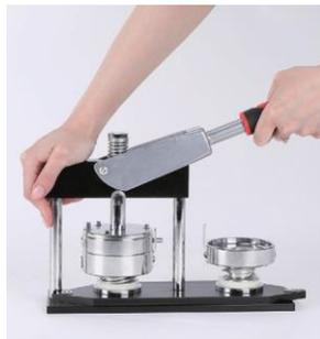
**15** Press the upper die down and hold it for 3 seconds as shown in the picture.
