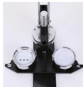
**10** Place the pin back into Mold B. Please note that the pin back and the patterned metal front should be facing away from each other.
