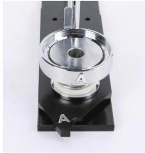
**3** Insert Mold A where A is marked.
