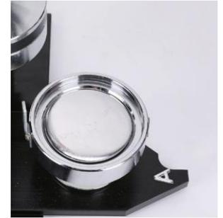
**6** Place the metal front into Mold A.
