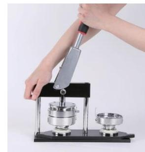
**11** Rotate Mold A beneath the upper die.
