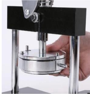
**2** Insert the upper die as shown in the picture, push it upwards and secure it.
