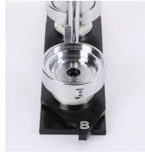
**4** Insert Mold B where B is marked as shown in the picture.
